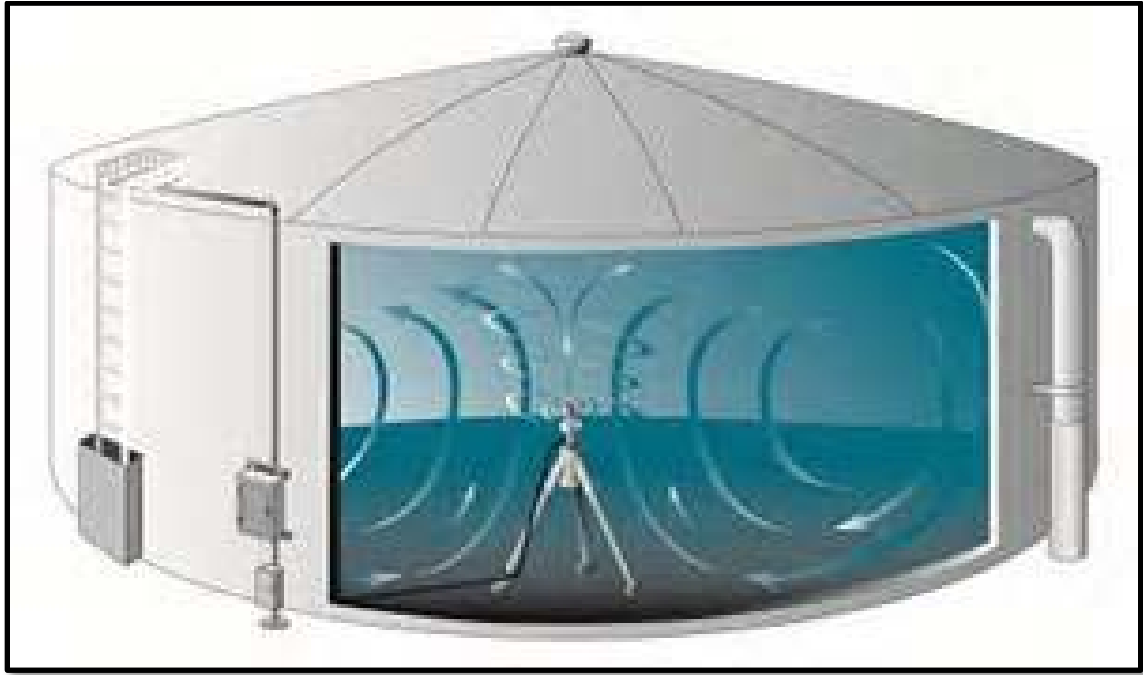
Sample Water Storage Tank Mixer Diagram
