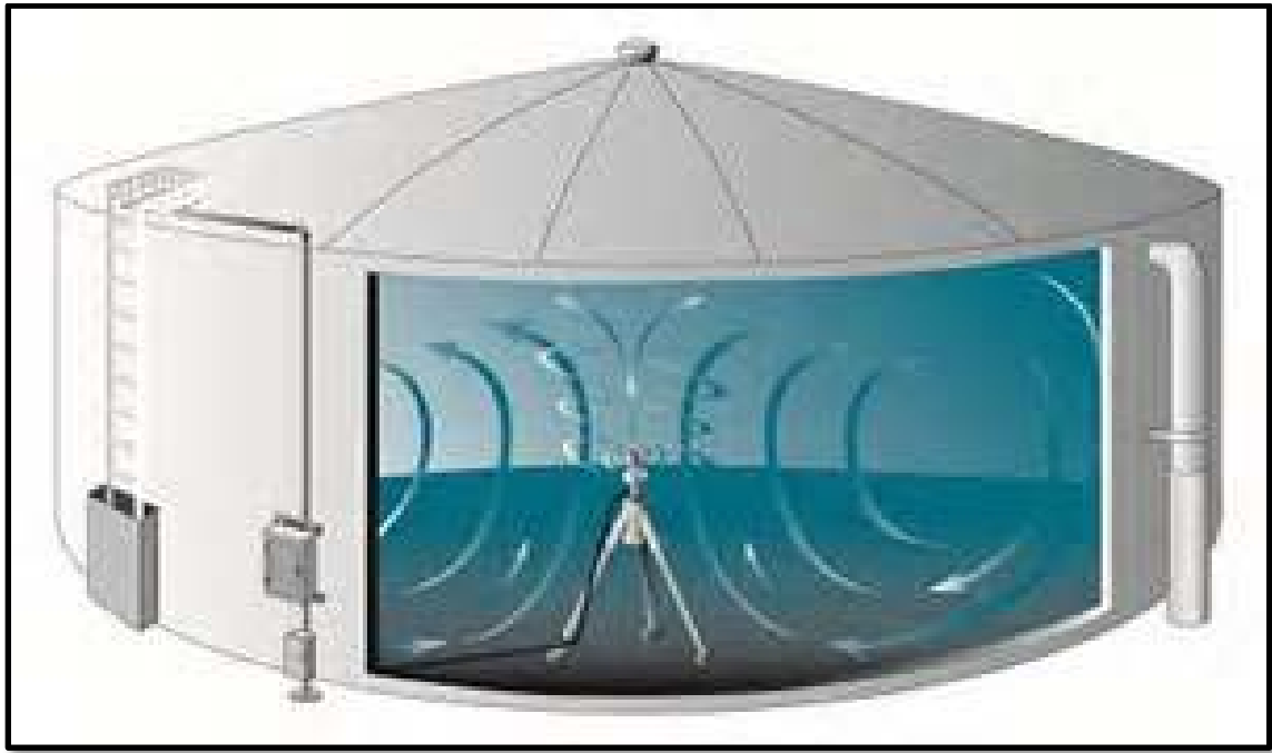
Sample Water Storage Tank Mixer Diagram
