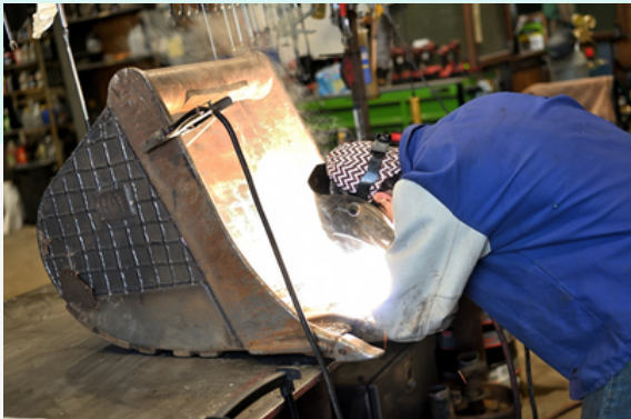
Tuker welds hard tac to the face of a backhoe bucket. A tried and true farmer repair that extends the life of contact faces on heavy equipment.
