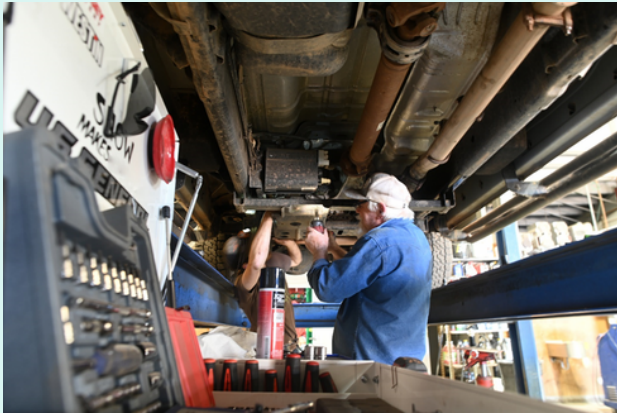
Chuck and Taker remove a transfer case for repair and re-installation all in the same day.
