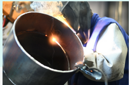
Tuker welds hard tac to the face of a backhoe bucket. A tried and true farmer repair that extends the life of contact faces on heavy equipment.
