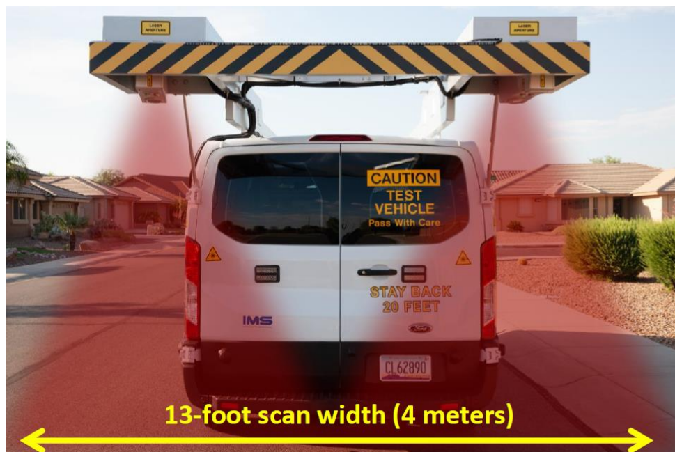
Figure 5 - RST Equipped with the 3D LCMS-2 Camera
